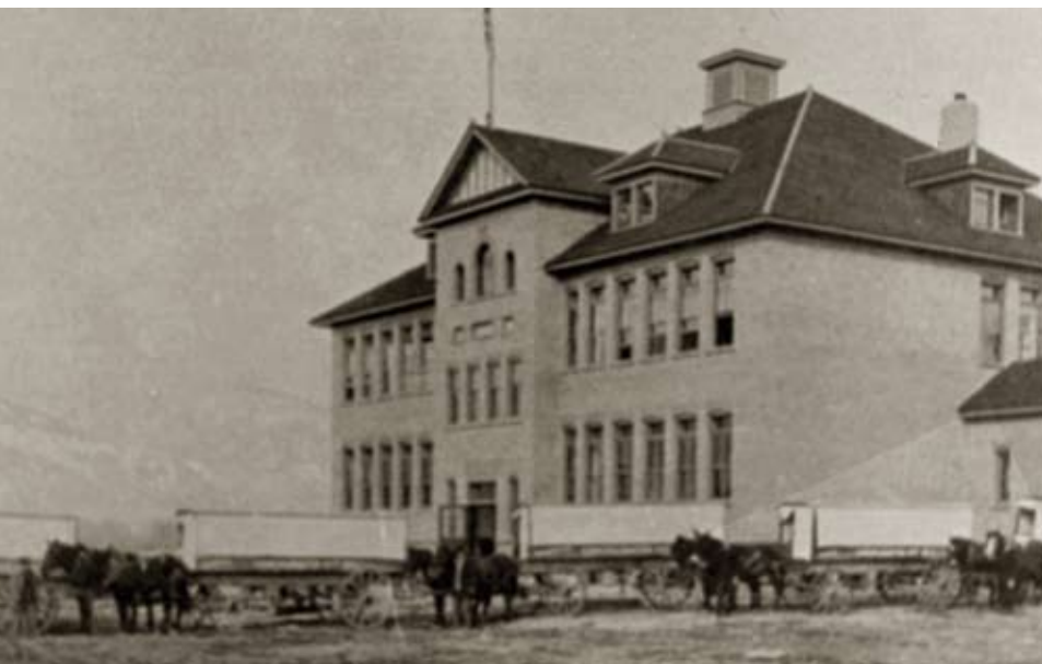
FIGURE 17.2: Did you ride a bus to school this morning? Students in Corvallis in the early 1900s rode to school in horse-drawn buses with canvas sides to protect riders from rain, snow, and road dust. Each wagon had a little coal stove so students could stay warm.
