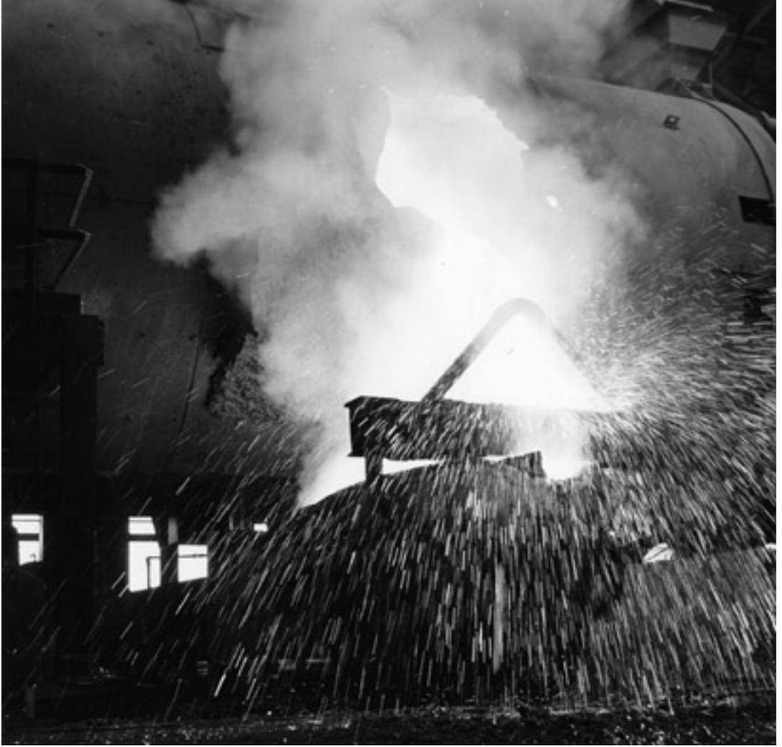
Russell Lee • Anaconda Smelter, Anaconda, September 1942. In this scene at the Anaconda smelter, molten copper being poured from the converter into the ladle splashed violently to make a dramatic photograph.
